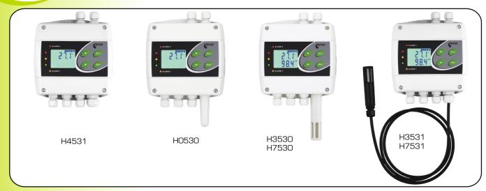
Transmitter is equipped with three binary inputs for detection of two-state events - e.g. water, smoke, glass break detection, door contact. Transmitter is equipped with internal terminals for powering of connected external detectors.
